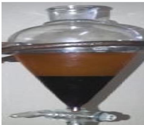
**Figure 2.3:-** Separation of biodiesel and glycerin as separate layers.
