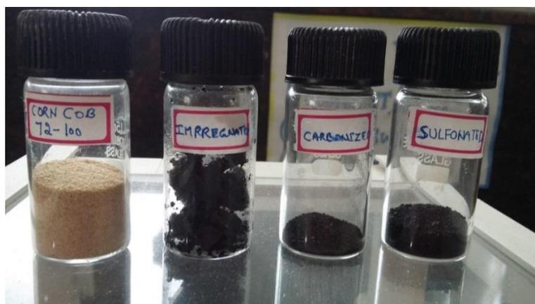
**Figure 4.1:-** Transformation of corn cob to the sulfonated catalyst.
