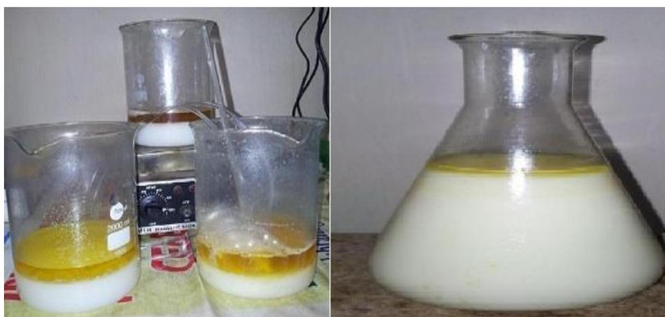
**Figure 2.4:-** Purification of biodiesel layer.
